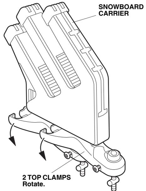
2. Install two board supports into the snowboard carrier.
